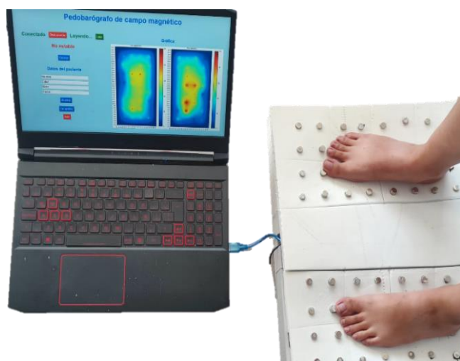
Fig. 3. Final pedobarograph of the magnetic field system with Hall effect sensors.
